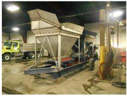
Past annual reports have failed to recognize the efforts of the men in the "shop". Howard Bair, chief mechanic is just one in particular. The hoppers used to blend our salt and stone for snow control has had over 89,000 tons of material ran through them since 1996 and the salt hopper finally rusted through. Instead of purchasing a new hopper, Howard built one out of stainless steel for \$16,000 less than what the manufacturer wanted for a mild steel bin.
